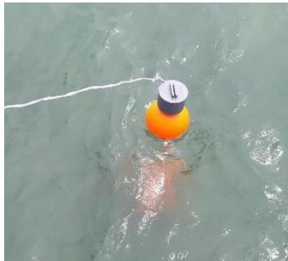
Gambar 4. Pengujian *drifter buoy*
